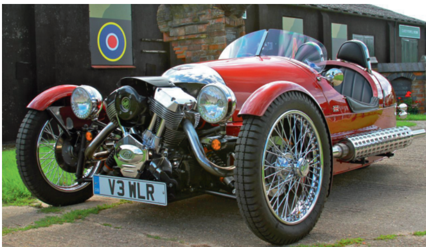
Figure 8 2013 M3W fitted with Garage56 exhaust and air filter. (Photo by Simon Goldsworthy)
